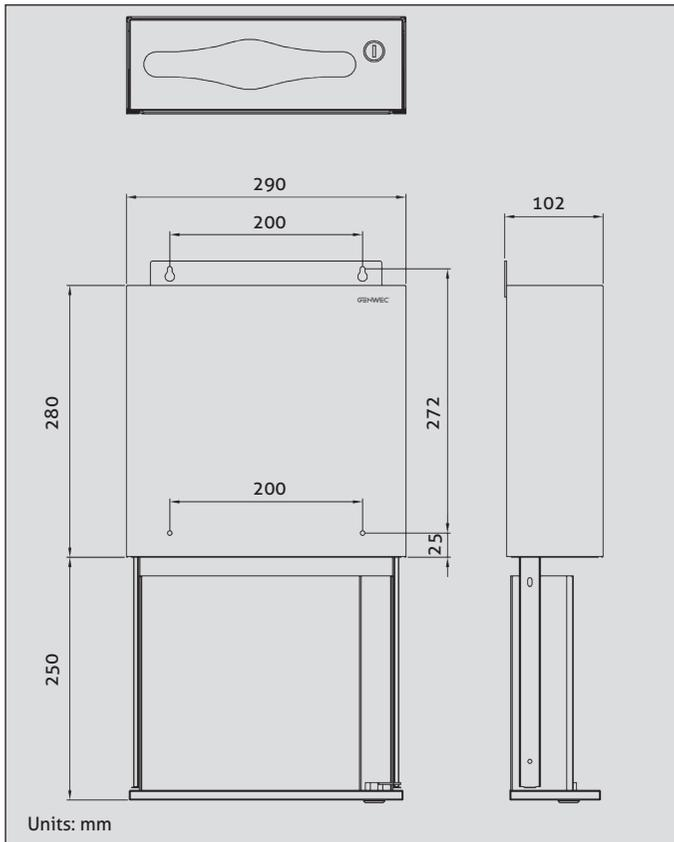
Insert the supplied nylon plugs. Then introduce the upper screws leaving 3-4 mm unscrewed.
