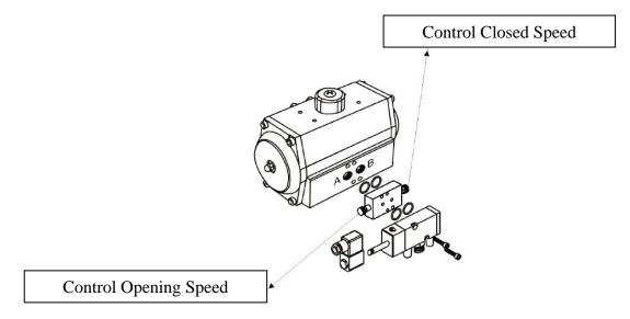
Verify that the o'rings are well placed on the back of the solenoid valve and speed controller and fix it to the actuator with the two screws that come in the box.
