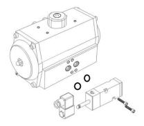
Verify that the o'rings are well placed on the back of the solenoid valve and fix it to the actuator with the two screws that come in the box.
