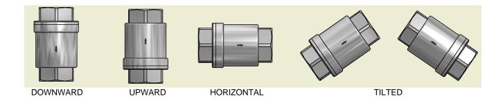
CAUTION: if the valve is installed without the spring, it must only be installed in a vertical position (upward flow).
