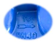
The trap must be installed with the buoy in a horizontal plane so that the movement is vertical, the arrow indicated on the cover indicate the installation position.
