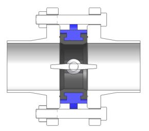
Fully open the valve before tightening the screws of the flanges
