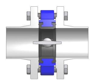
Leave enough space between the flanges so that valve can be easily inserted or removed
