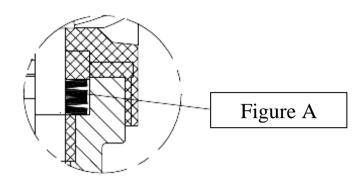
c.- Replace the Disc (part. 6) in its working position within the seat (part. 5) proving it has not been damaged during the disassembly process and aligning the holes in the disc with the holes in the seat.
