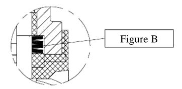
f. - Place the lower body (part 1) in all pre-assembled, matching the marks previously made in the body parts to keep its original position.
