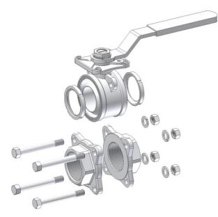
b.- Loosen and remove the 4 / 12 *nuts* (part. 20 / part. 22 Art.2933) of the *screws* / *bolts* (part. 18 / part. 20 Art.2933) that bring together the three different parts of the valve. Remove the screws.
